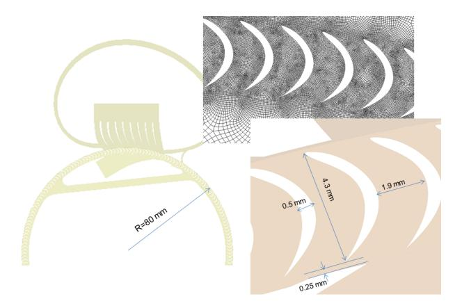
Figure 8. Two-dimensional mesh and geometry developed for steady-state and transient sumulations
