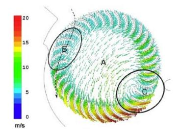
Figure 3. Three characteristic flow zones in cross flow blower. Source: Dang and Bushnell (2009)
