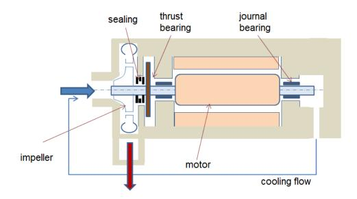
Figure 4. The reference compressor concept
