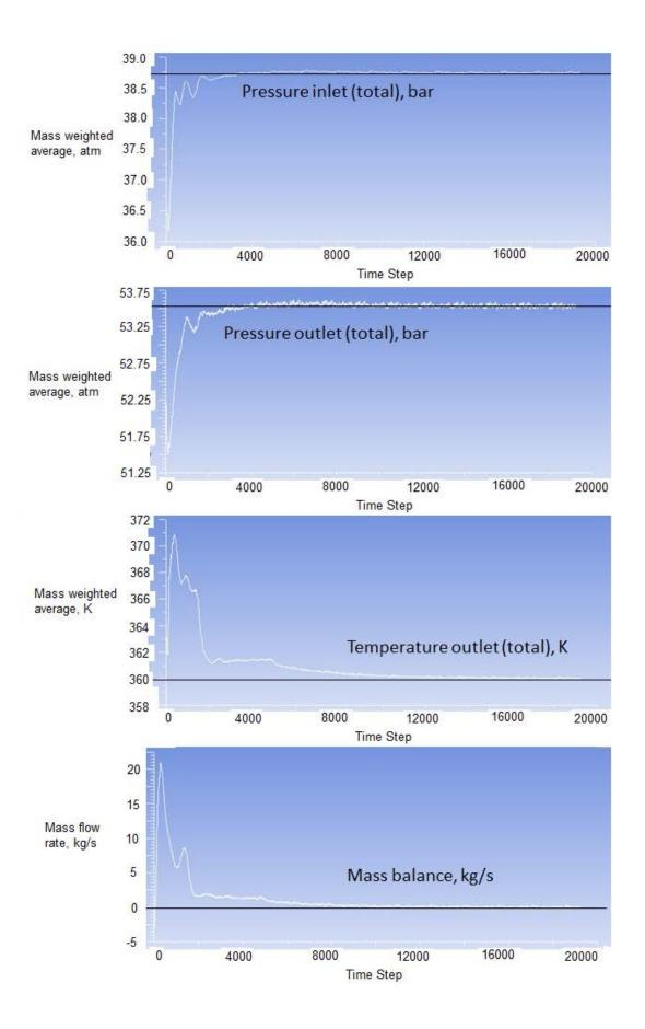
Figure 9. Main monitors' history of the transient simulation
