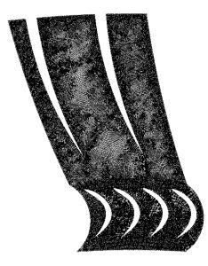
Figure 14. The meshed domain of 1/50 of the full wheel depicting the reference blade shape
