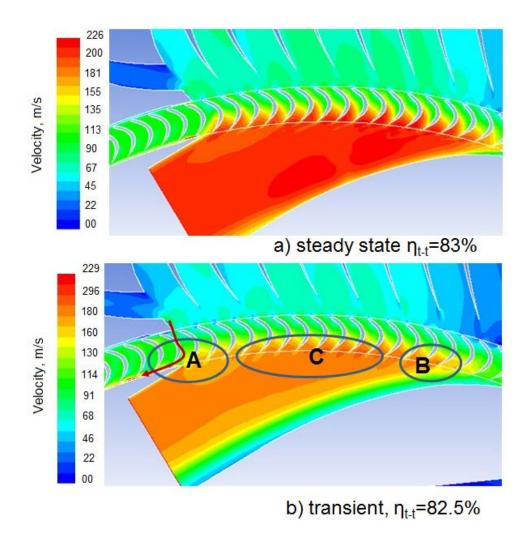
Figure 10. Comparison of velocity field obtained by steady-state and transient CFD analysis
