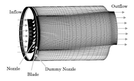
Figure 1. Numerical grid for simulation of partial admission axial steam turbine. Source: Sakai et. al.
